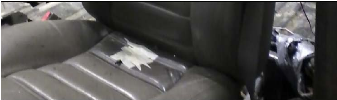
FIGURE 3: The temperature sensor in position and taped to the top of the seat to detect body heat.
