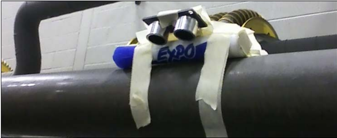
FIGURE 4: The ultrasonic range sensor mounted to the exposed frame of the Hummer as well. It was positioned above the seat at a slight angle to measure the height of any occupant.
