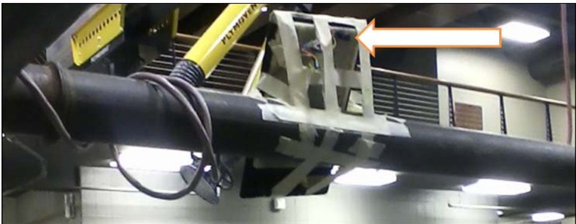
FIGURE 5: The passive infrared occupancy sensor was positioned in front of and above the seat, angled downward. It was mounted on the exposed frame of the Hummer. The arrow in the figure points to the actual sensor which is in a breadboard to make the position more stable.
