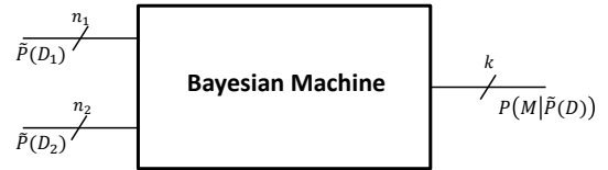
Fig. 1. Simple Bayesian Machine with two inputs and one output, and no free variables. The compilation toolchain takes a Bayesian program specification and uses ProBT to have a symbolic description of the computation used to synthesise the machine.
