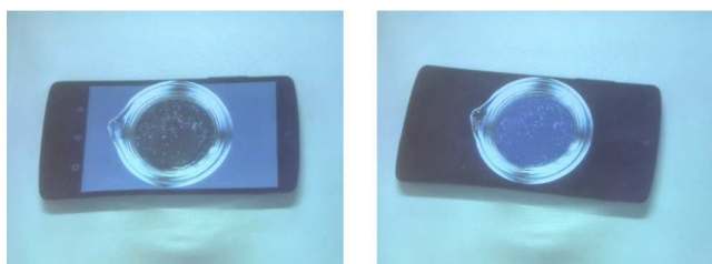
15 16 Figure 2: A dilute solution of sucrose exhibiting a rotation of ca. 5^\circ . The phone was rotated to minimize light from the screen (right) and the 17 sample (left). A video of this in action is available in the Supporting Information. 18
