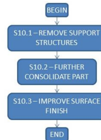
Figure 16: "Manufacturing: Post Processing" Flowchart
