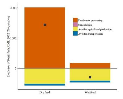
**Figure 3.5 – Fossil fuel use (MJ) in the production of wet feed and dry feed.** The processing stage for dry feed has much higher fossil fuel use than wet feed because of the additional dehydration of food waste during production. Both avoid fossil fuel use associated with the production of conventional pig feed. The black points mark the net fossil fuel use per technology.
