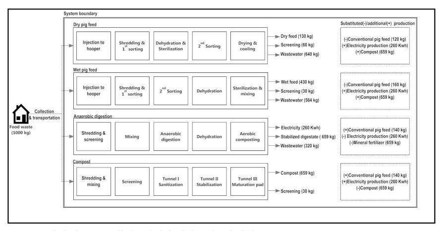
Figure 3.1 – Steps involved in the processing of food waste by the four food waste disposal technologies. Only major material flows are shown: minor inputs (e.g. water, corn in the case of wet feed) and evaporation are not included for the sake of clarity. Outputs are indicated by arrows and substituted products are shown in the boxes on the right-hand side. Mineral fertilizer substitution rates of digestate and compost are listed in section 2.1.3 and Appendix J, Table 9-8, respectively.
