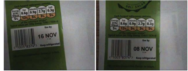
Fig. 9. Example of OCV classification. On the left hand side, a label whose use by date is relatively easy to be identified. On the right hand side, the proposed algorithm was able to recognise (in the experiment 5 vs 8) the correct day (8) despite the presence of several 5's across the image.
