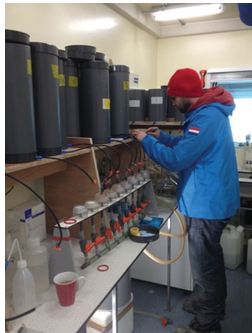
Fig. 11. Lab 2: used for processing water samples and performing biological rate measurements at the temperature of the sample of interest (0–15°C). Photo: R. Visser
