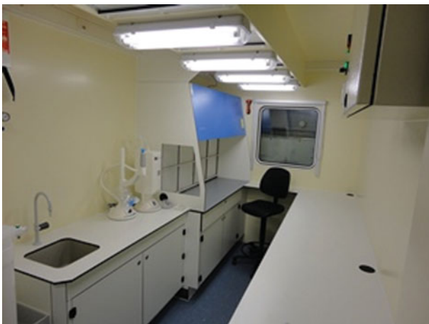
Fig. 13. Lab 4: a clean room suitable for trace metal analysis and for measuring low concentrations of contaminants. It is equipped with special filters in the air processing system and is free of (uncoated) metal. Photo: H. de Porto
