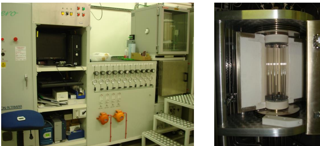
Figure 2.13 Oxidative dehydrogenation testing rig, (left) photograph of rig, (right) photograph of sample container.
