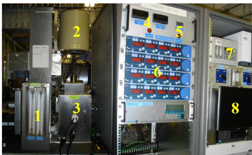
Figure 2.9 Photograph of the Transient 2 rig showing (1) FTIR and Bypass flow meters, (2) Furnace, (3) Sample oven, (4) IN/OUT pressure transducers, (5) Heated rotameter enclosure (6) MFC control panel, (7) Oxygen analyser, (8) Micro GC monitor.
