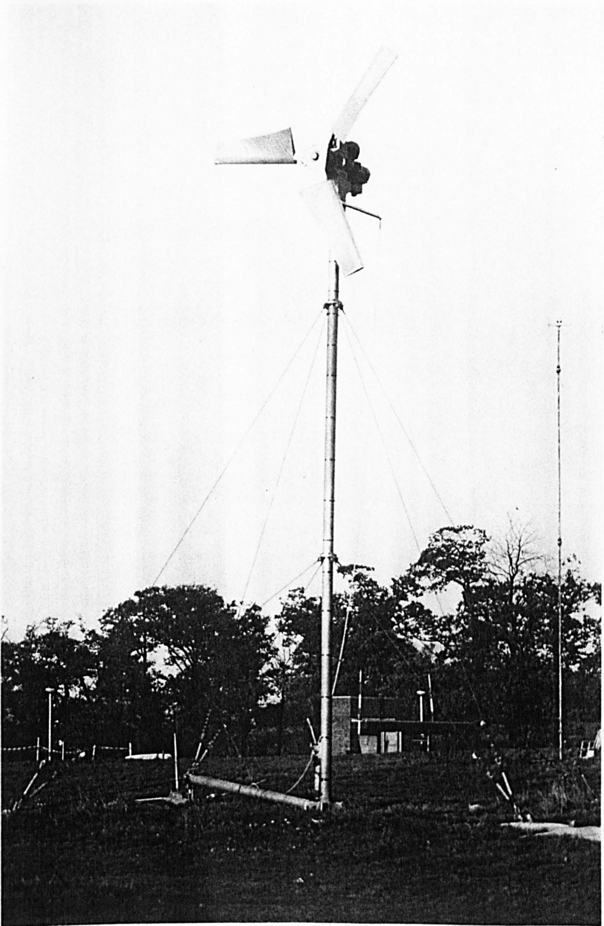
Fig 9.14: ATG 4m Dia Sailfoil HAWT under test on ATG Wind Turbine Test Facility
