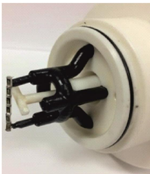
Figure 4. Components of the measurement cell including on-board resistors and stirring paddle.
