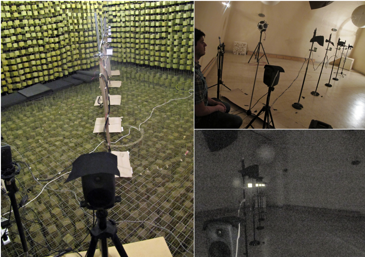
Figure 1: Details of the experimental setup. (a) View from above the subject in the anechoic room. (b) Lateral view in the reverberant room. The subject can be seen on the left. (c) View from the subject position in the reverberant room. The room is in darkness and all targets are lit. The shot was taken with a little displacement to the right, in order to avoid occlusion by the nearest targets.
