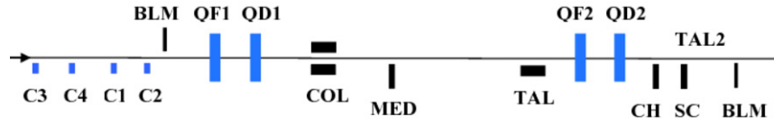
Fig. 1. (Color online.) The modified layout of the UA9 experiment. The primary collimators – bent crystals C1–C4 are located upstream the quadrupole QF518 (QF1). The TAL acting as a secondary collimator–absorber is upstream the quadrupole QF 520 (QF2). The TAL2 station in a high dispersion area is used to measure off-momentum particles produced in the collimation process.
