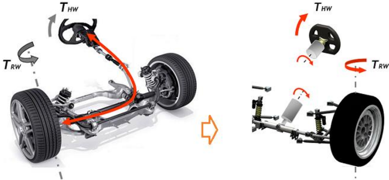
Figure 1 – Differences between conventional mechanical steering arrangement (left) and SbW System (right)
