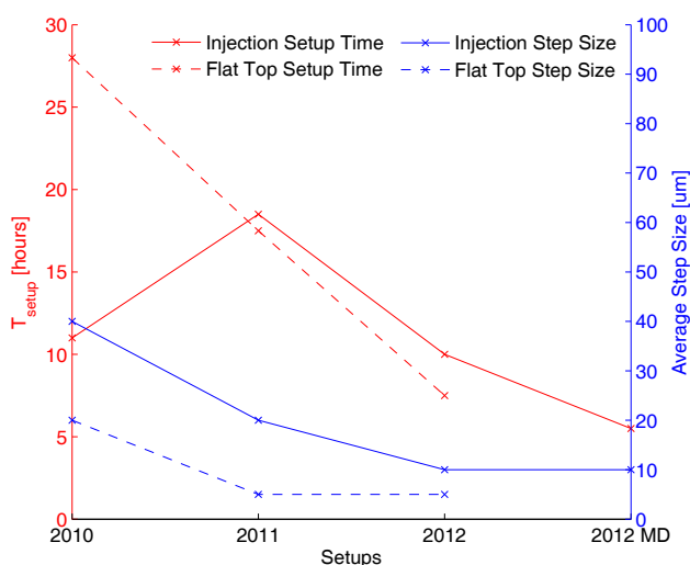
Figure 6: Evolution of the setup time for the collimator alignments and the average jaw step sizes used at injection and flat top from 2010 to 2012. The 1 hour 45 minutes required to setup 27 collimators during the 2012 MD is extrapolated to 5.5 hours for a full setup.
