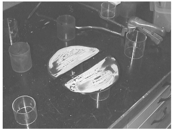
Figure 2 – Drying of Copper Nitrate on the back of the sample.
