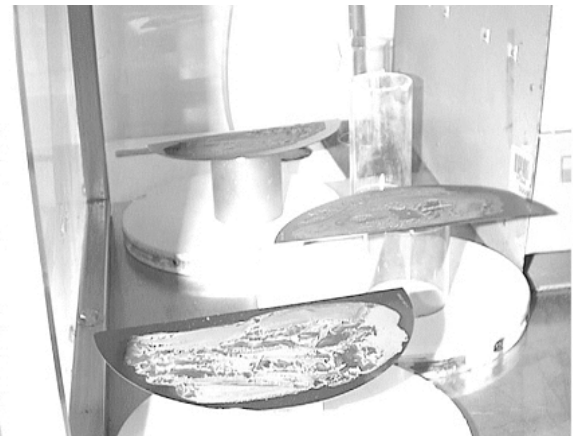
Figure 2 – Drying of Copper Nitrate on the back of the sample.
