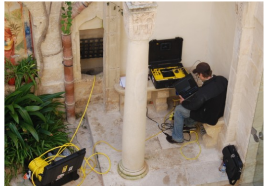
Figure 2: A typical ROV deployment in which the robot is driven by computer, while video feedback is recorded and maps are constructed with sonar data. Note the yellow tether descending into the mouth of the access point. The photo was taken in the Palazzo Falzon courtyard, Mdina.
