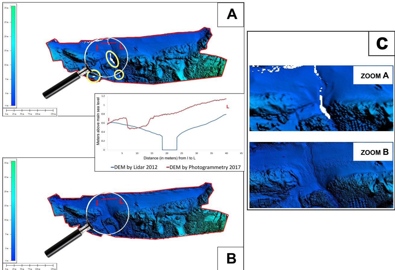
**Figure 7:** LiDAR DEM (A), Photogrammetric DEM (B), comparison between zoomed areas on LiDAR DEM and photogrammetric DEM.
