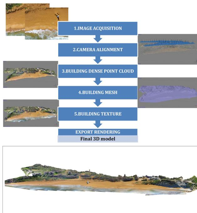
**Figure 4:** Workflow processing to obtain the final 3D model.
