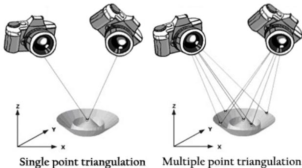
**Figure 1:** Schematic triangulation processes for photogrammetry.
