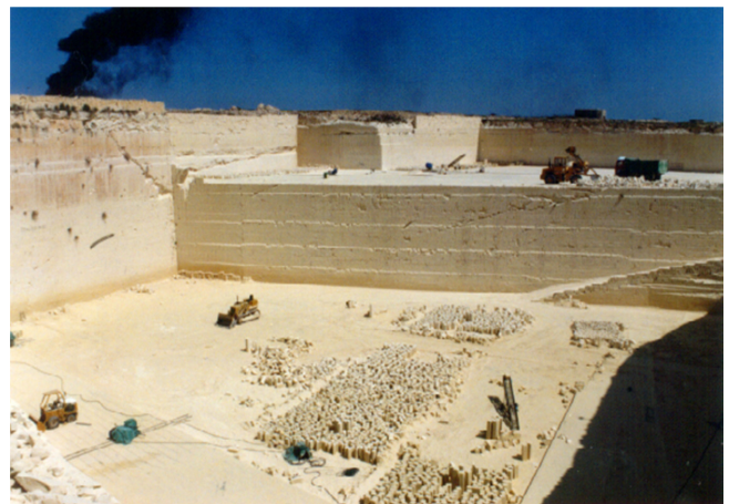
Figure 3. Open pit quarry extraction in the quarry area of Mqabba, Malta. Extraction is by automated sawing machines. Processing starts in the quarry and continues on site.
