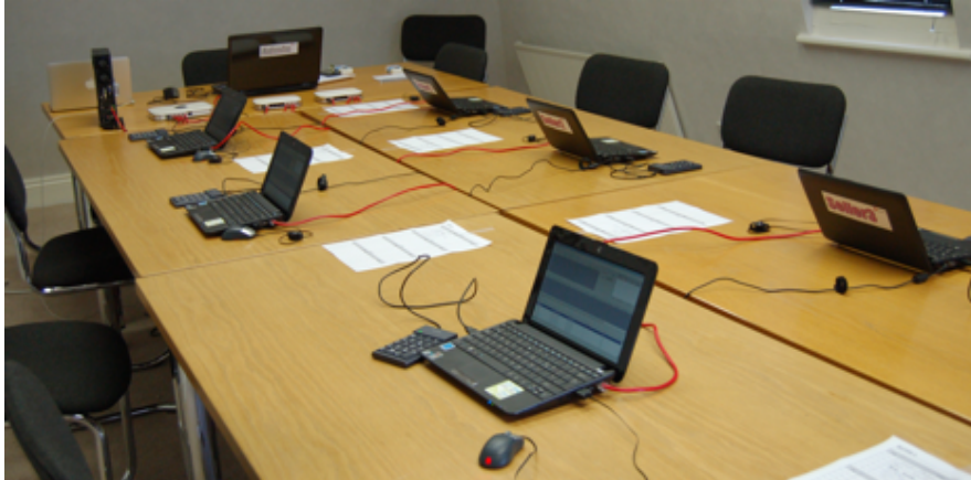
Fig. 2 The Lab-in-a-box hardware ready to run an Open Exchange (OpEx) human versus agent trading experiment. Six small netbook computers run human trader Sales GUIs, with three buyers (near-side) sitting opposite three sellers (far-side). Net-book clients are networked via Ethernet cable to a network switch for buyers and a network switch for sellers, which in turn are connected to a router. The central exchange and robots servers run on the dedicated hardware server (standing vertically, top-left), which is also networked to the router. Finally, an Administrator laptop (top table, centre) is used to configure and run experiments. Photograph: © J. Cartlidge, 2012.
