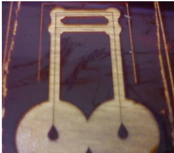
Figure 4.5 AZ mould for PDMS microfluidic channel fabrication
