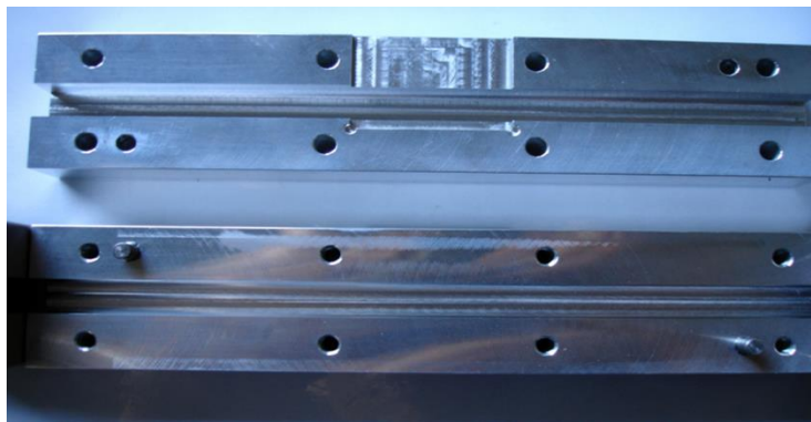
Figure 5.5 Picture of modified waveguide to accommodate the thickness of PMMA channels
