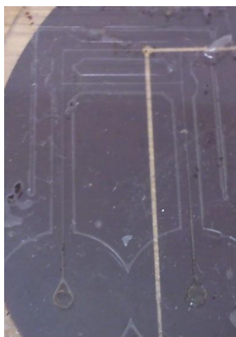
Figure 4.7 Completed PDMS structure
