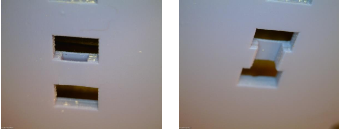
Figure 8.4 Left: closed; right: open LTCC cavity using silicone as a sacrificial material
