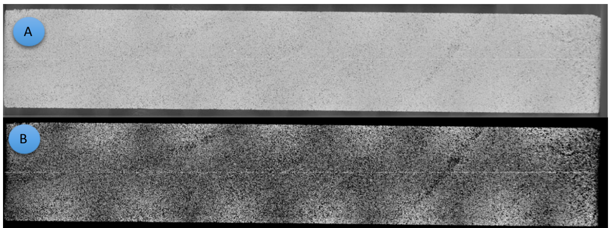
Figure 4-4 CT-Scan results of the heterogeneous sandstone core (30 cm*4.9 cm)
