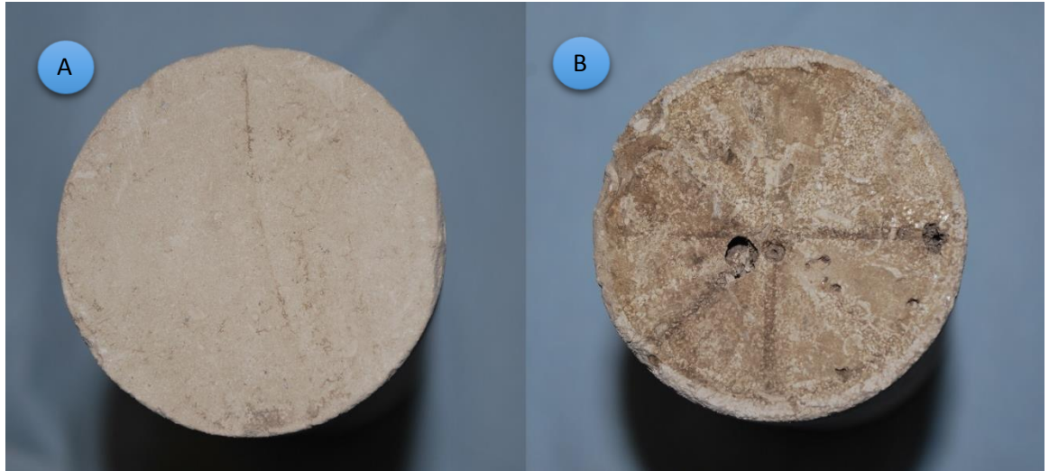
Figure 5-4 Inlet of a reservoir carbonate core A) before and after B) CWI
