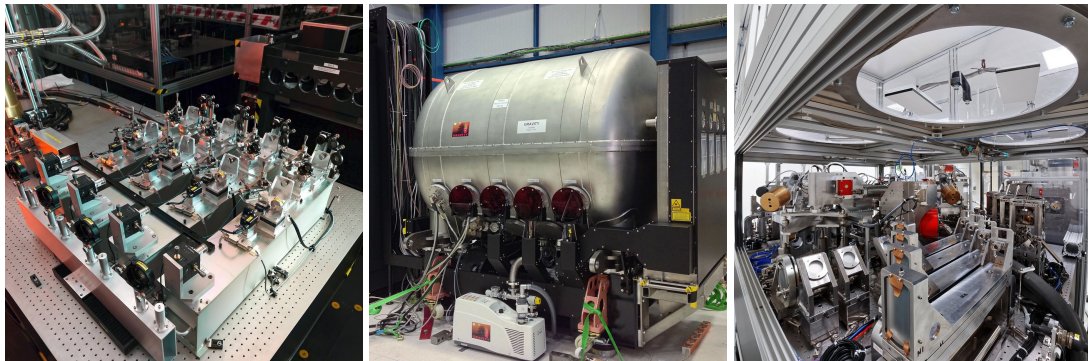
Figure 2: From 2019 the VLTI interferometric instruments will cover the full atmospheric windows H-band to N-band (1.6 - 13 micron): left: PIONIER (H-band; in regular operation), center: GRAVITY (K-band; 2016 in commissioning at the VLTI), right: MATISSE (L, M, N-band; photo taken in the lab; VLTI commissioning will commence in early 2018). Image Credits: ESO, B. Lazareff, MPE/GRAVITY team, MATISSE project, Y. Bresson.
