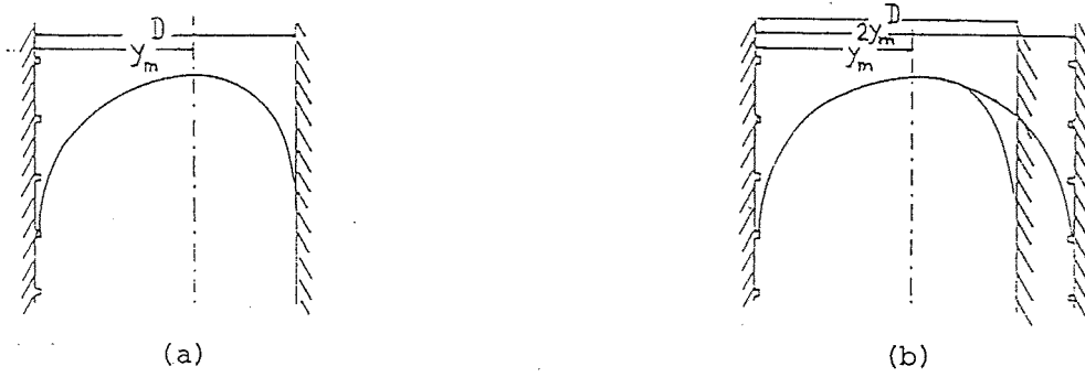
FIGURE 2.1 Schematic presentation of the Hall transformation theory: (a) the real rough channel; (b) the "equivalent" rough channel.
