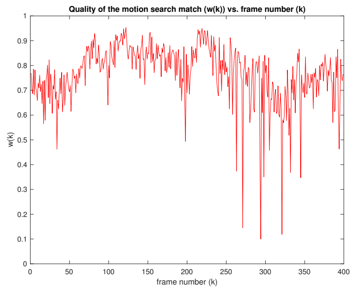
Fig. 5.16 Inter-frame registration weighting for the pipeline and pile dataset.
