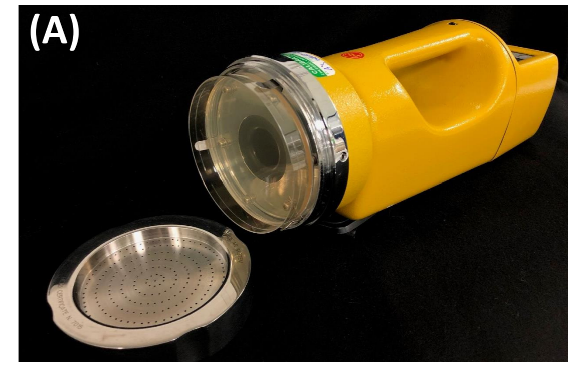
Fig 1. (A) SAS Super 180 Impactor air sampler with fitted TSA plate and separate aspirating head and (B) ICU patient isolation room layout showing position of air sampler.
