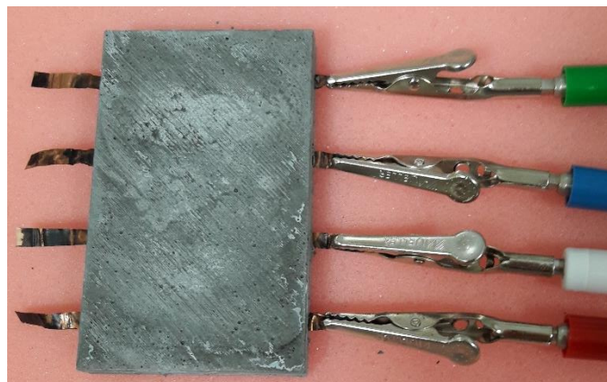
Figure 4. A four-electrode EIS cell with a geopolymer samples and copper electrodes
