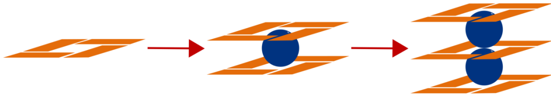
Figure 1-7 Schematic showing how the stacking of guanine tetrads is mediated by monovalent cations. The orange quadrilaterals represent the guanine bases of the tetrad and the blue circles represent the monovalent cations.
