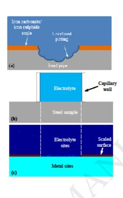
Fig. 9 Schematic of cellular space for cellular automata modelling.
