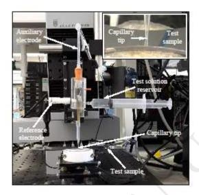
**Fig. 2.** Schematic of experimental set-up of scanning droplet cell and fatigue test rig for investigating the effect of stress and electrolyte flow on localised corrosion.
