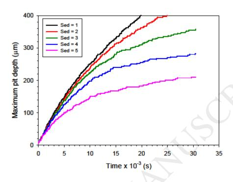
**Fig. 17.** Influence of metal ion hydrolysis on time-dependent evolution of maximum pit depth (The coloured version of this figure is available online).
