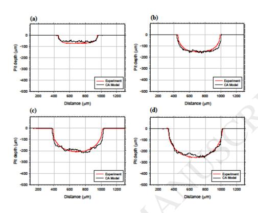
**Fig. 15.** Influence of metal oxidation on time-dependent evolution of maximum pit depth (The coloured version of this figure is available online).
