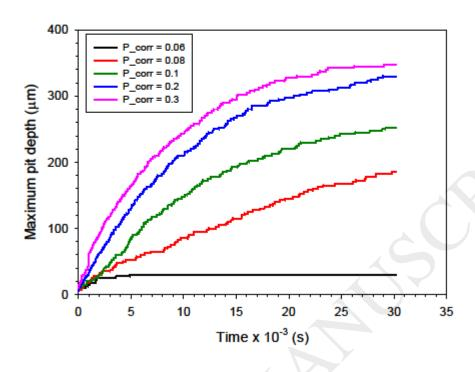
**Fig. 16.** Influence of corrosion products accumulation on time-dependent evolution of maximum pit depth (The coloured version of this figure is available online).
