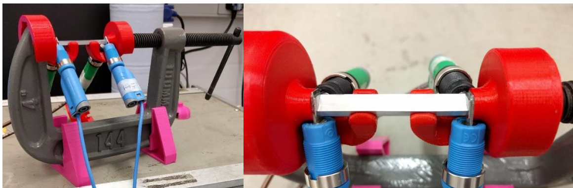
Figure 2: Electrical test jig and setup showing polished aluminium test sample clamped between four-wire Kelvin probes.
