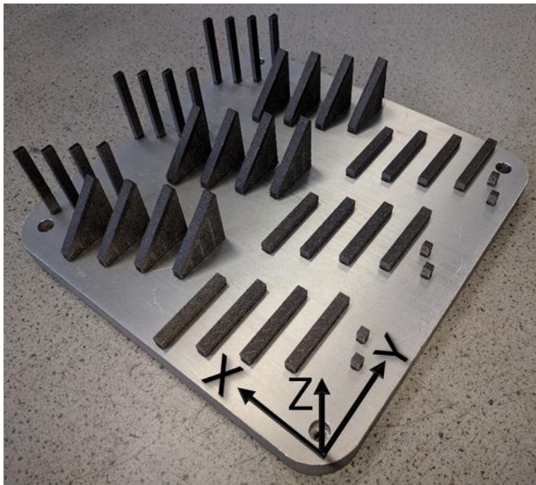
Figure 1: Build plate with electrical test bars printed in vertical, 45-degree, and horizontal initial build orientations along with 5mm sample cubes.
