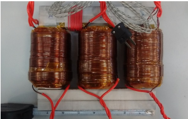
Fig. 8. A 10kW/1kHz prototype of 3DAB transformer
