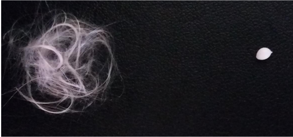
Figure A7. Photos of the glass wool before (left) and after (right) calcination at 800°C.
