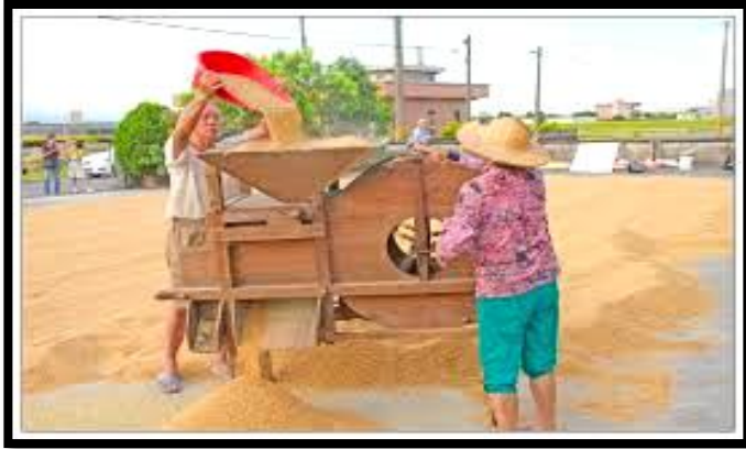
Winnowing rice with a simple hand machine. Photo credit: Sophia Kashenge/ ARI Dakawa.
