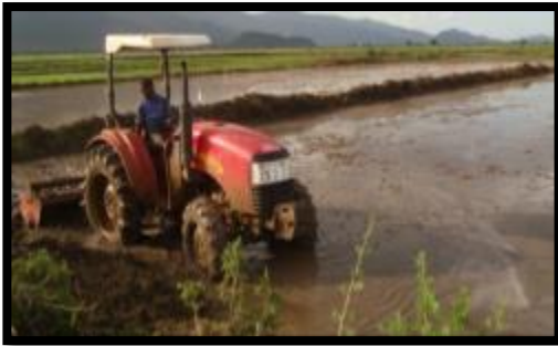
Soil puddling using a tractor-drawn rotorvator. Photo credit: Ndimubandi Mvukiye/ARI Dakawa.
