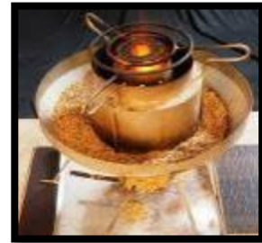
Different cooking stoves using rice husks as fuel. Photo credit: Ndimubandi Mvukiye/ ARI Dakawa.
