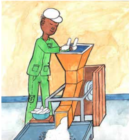
Figure 10.1 Grating cassava using a mechanized grating machine
