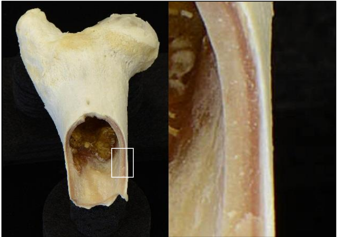
Figure 7.27: Proximal fragment of a high pH sample fractured after two exposure periods (left) and close up of the fracture surface (right) showing the variation in opacity and colour across the thickness of the cortical bone (source: author).
