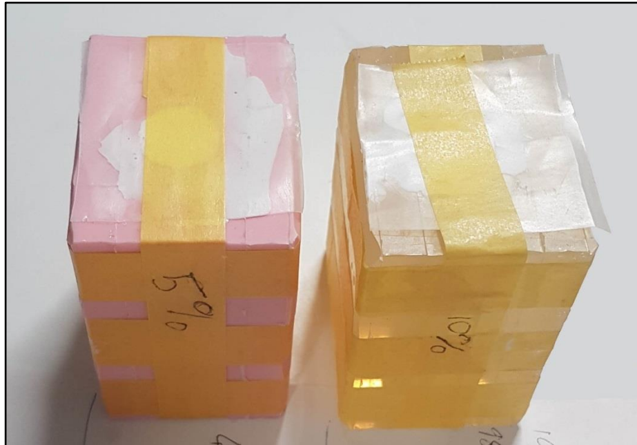
Figure 5.23: Casting the opacity technique comparison standards with 5% and 10% opacifier into the RTV silicone moulds (source: author).
