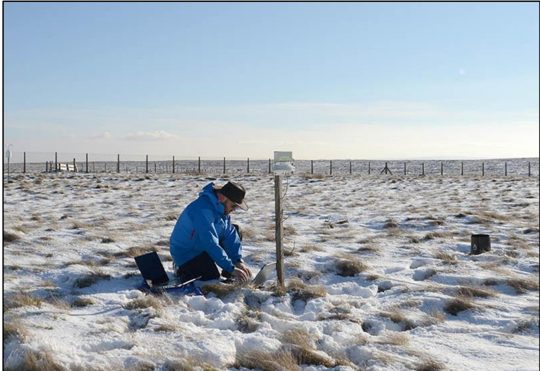
Figure 5.4: Downloading weather data from the Helios weather station in February 2015. Rainfall is measured by the black rain gauge bucket on the right of the image, all other readings are contained in the instrument's white housing atop the wooden pole (source: author).
