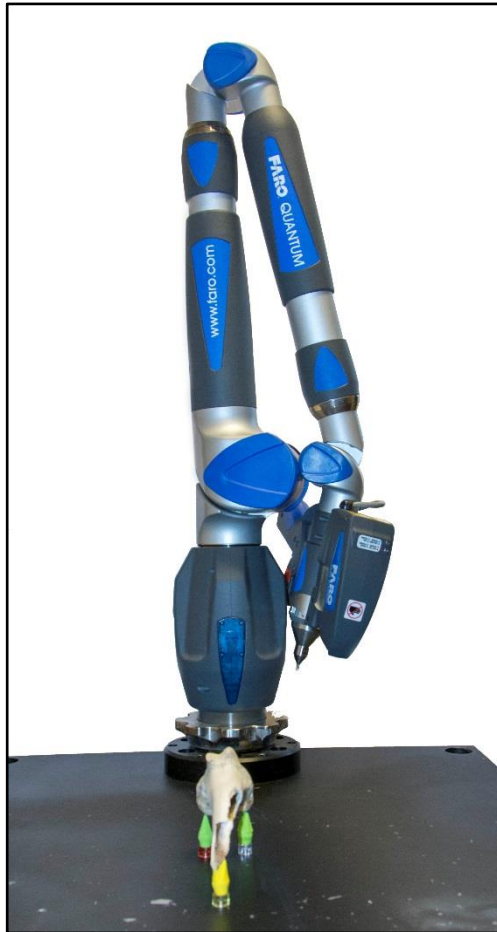
Figure 6.1: FARO Quantum Arm with V3 Laser Line Probe mounted on a Bradford Visualisation metrology instrument bench (source: author).
