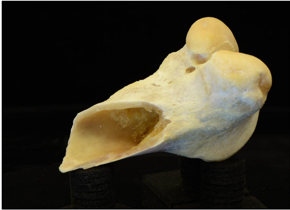
Figure 7.26: Fracture surface of a high pH sample fractured after the first exposure period showing the sharper fracture margins and the variation of colour and opacity across the exposed cortical thickness (source: author).
