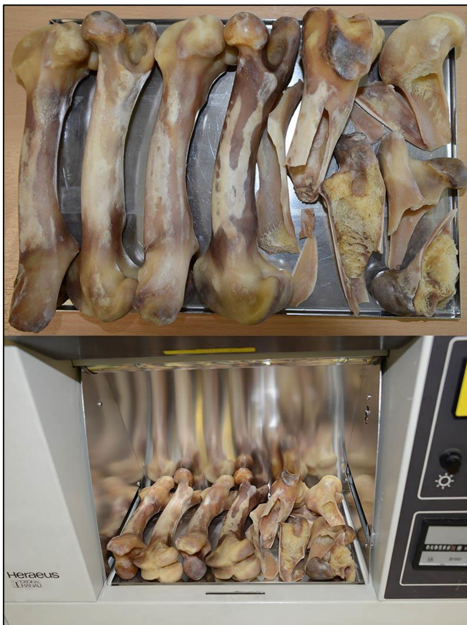
Figure 5.10: Bone samples placed on the stainless steel exposure tray prior to exposure (top) and with the exposure tray inside the Heraeus Suntest CPS unit (bottom) (source: author).
