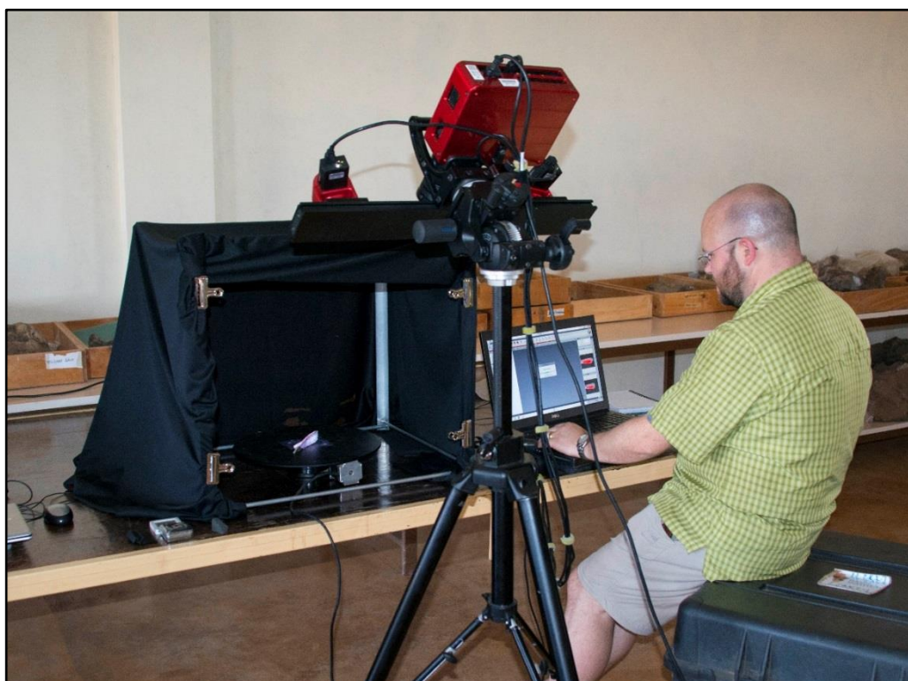
Figure 5.14: MechInnovations MechScan macro structured light scanner as set up in the Turkana Basin Institute's Ileret field centre laboratory (source: author).
