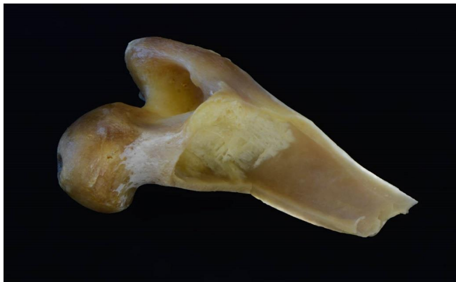
Figure 7.33: Fracture surface of high UV sample fractured after the second exposure period showing the increased opacity from photodegradation of the outermost layers of the cortical bone in the fracture surface outer margins (source: author).
