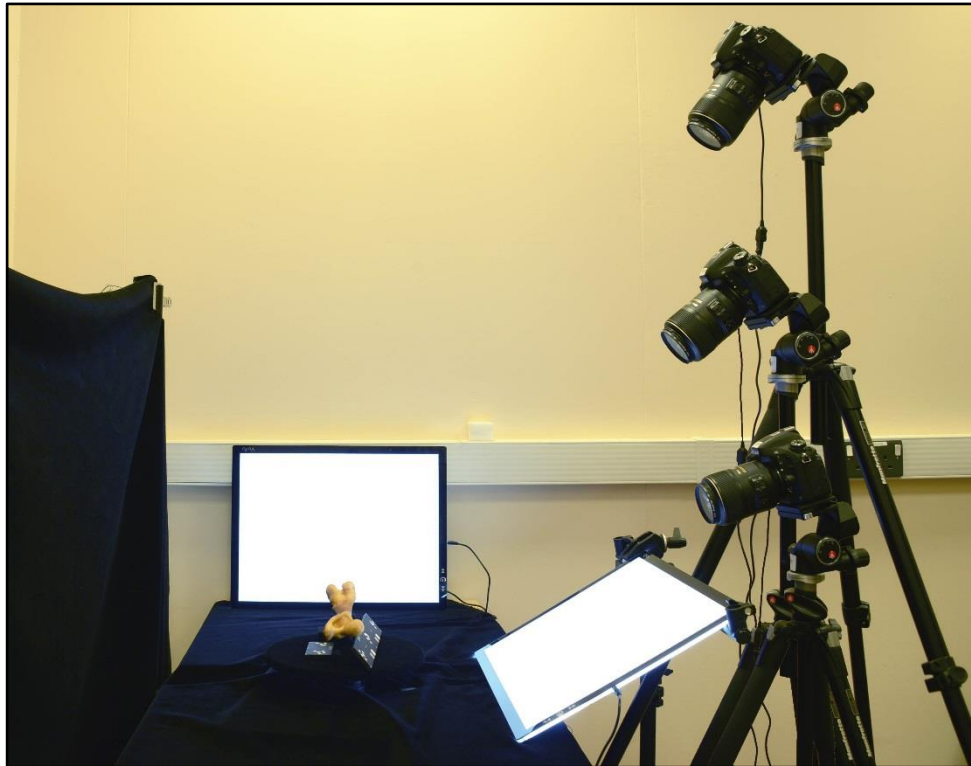
Figure 6.14: Composite image showing the three camera positions used in the photogrammetric recording within the Bradford Visualisation photographic suite (source: author).
