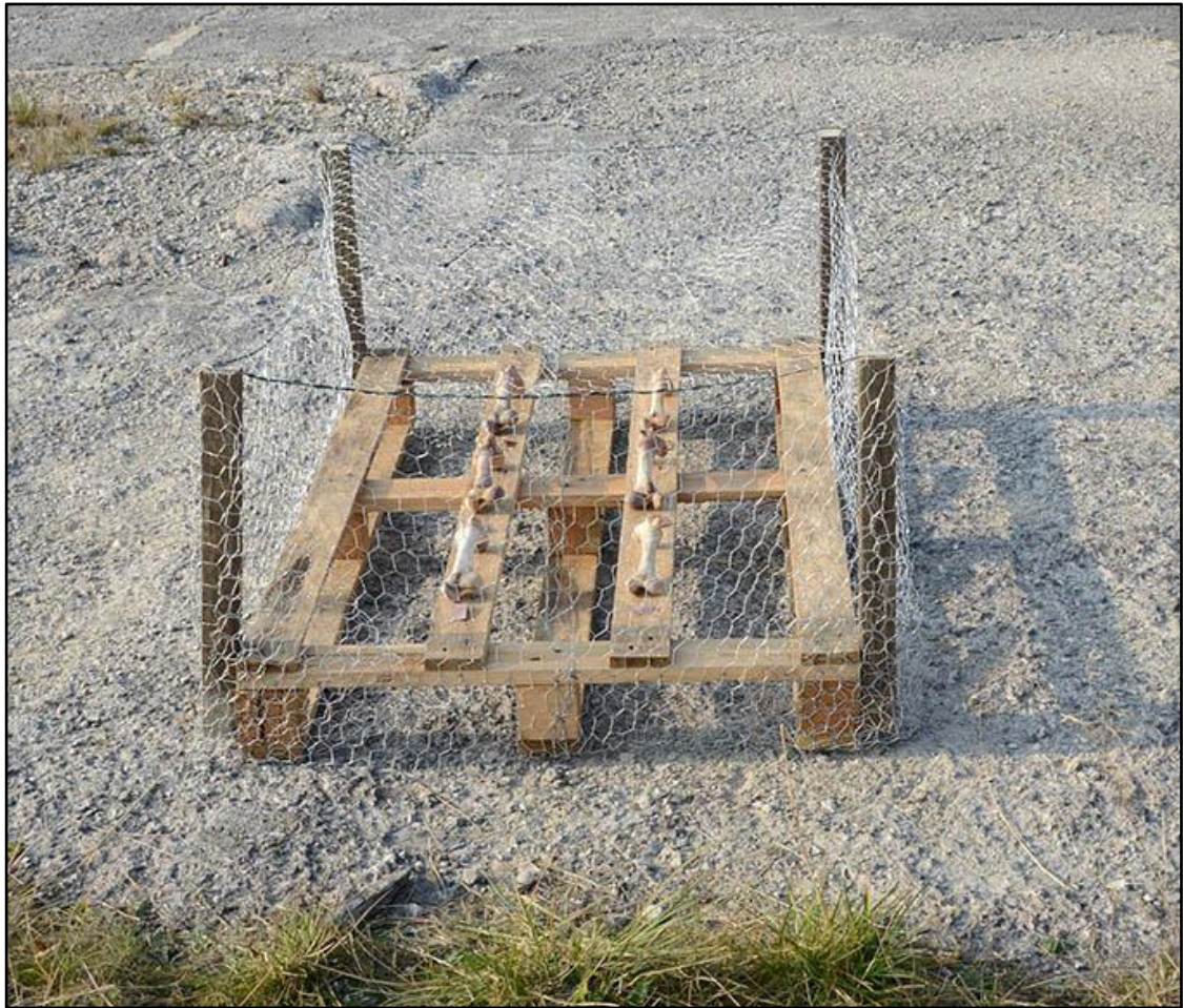
Figure 5.3: Weathering samples within the wire cage to protect from predation (source: author).
