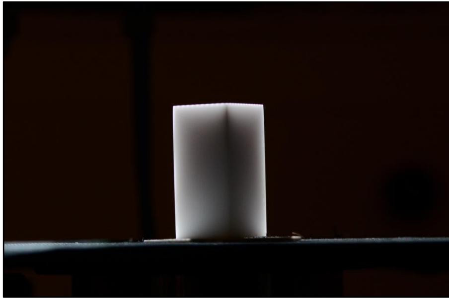
Figure 8.3: Photo of edge transmittance of light in opacity sample S0011 photographed during structured light scanning lit from behind by the structured light scanner as the light source (source: author).
