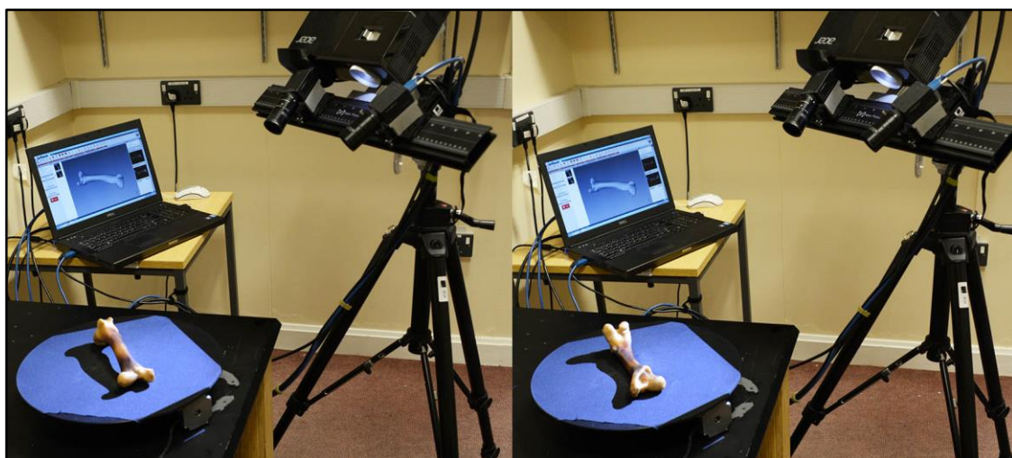
Figure 6.7: Sample A0021 on the structured light scanner turntable in anterior (left) and posterior (right) orientation (source: author).
