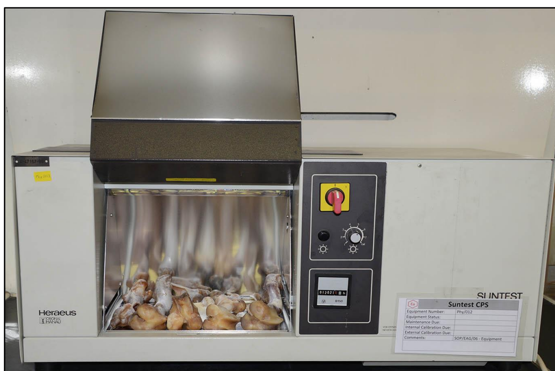
Figure 5.8: Heraeus Suntest CPS benchtop xenon UV and visible light exposure unit (source: author).
