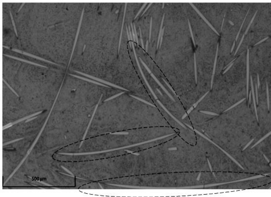
Figure 2.21 Example of curved fibres in a long glass fibre sample
