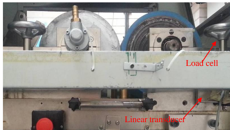
Figure 3-2 The experimental rig, feed & deformation control (gap & load) [120]
