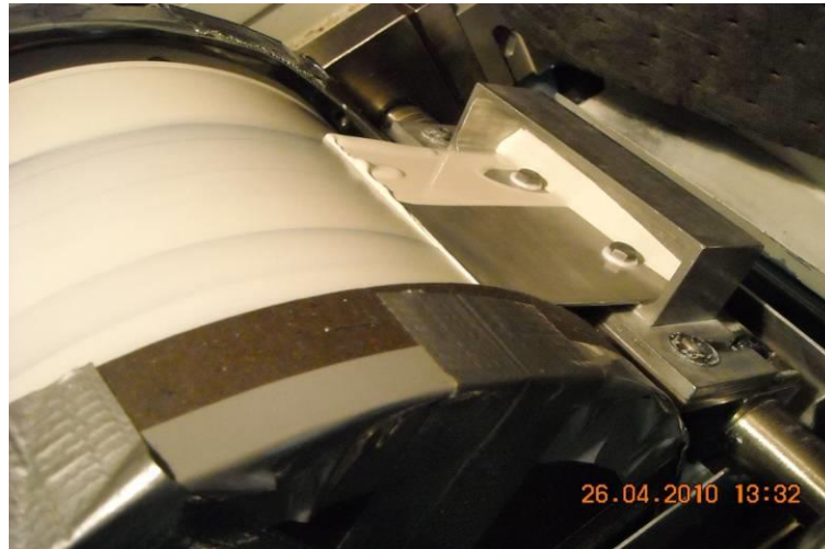
Figure 3-16 Non uniform scrapping with aluminium scrapper
