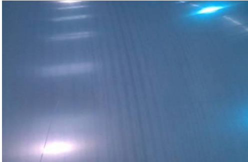
Figure 5-53 Ribbing on steel substrate
