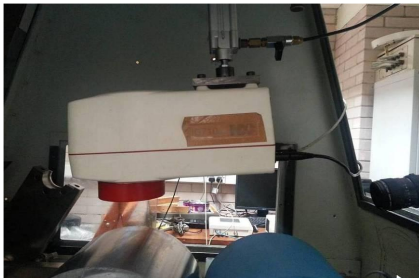
Figure 3-19 Non contact wet film thickness (WFT) instrument in coating rig
