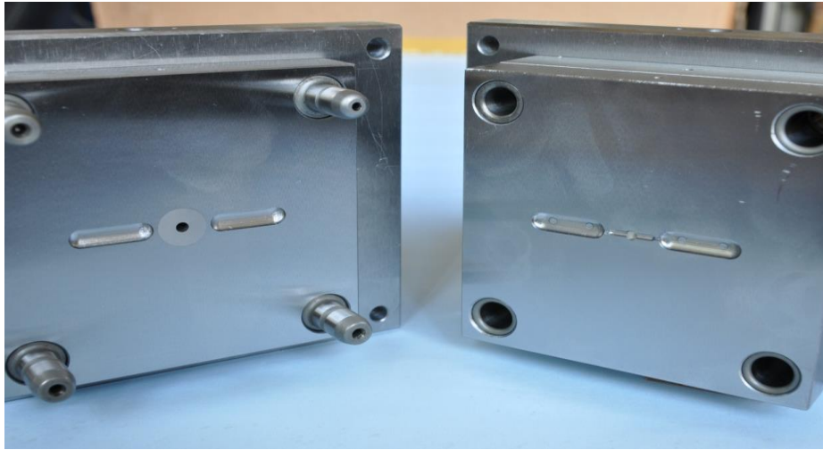
Figure 3.6: FANUC Roboshot i5A injection moulding machine, tensile bar and tablet mould design
