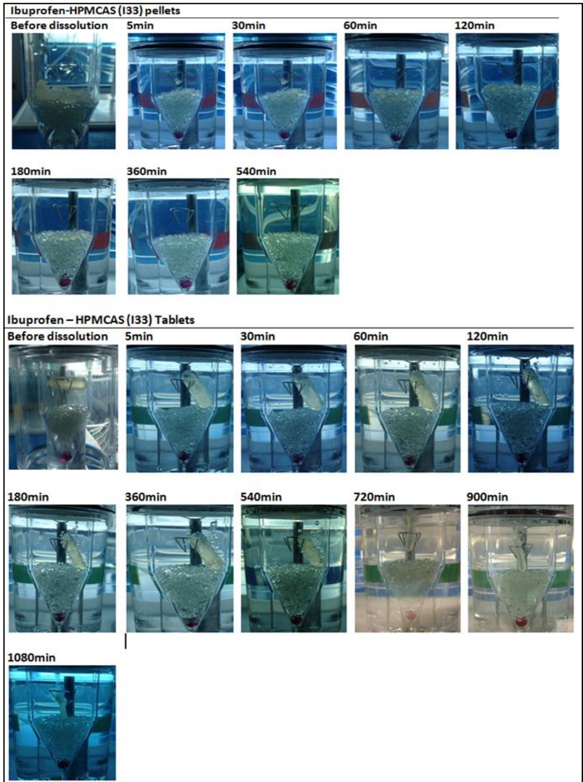
Figure 5.78: Dissolution images of I33 pellets and I33 moulded tablets (USP IV)
