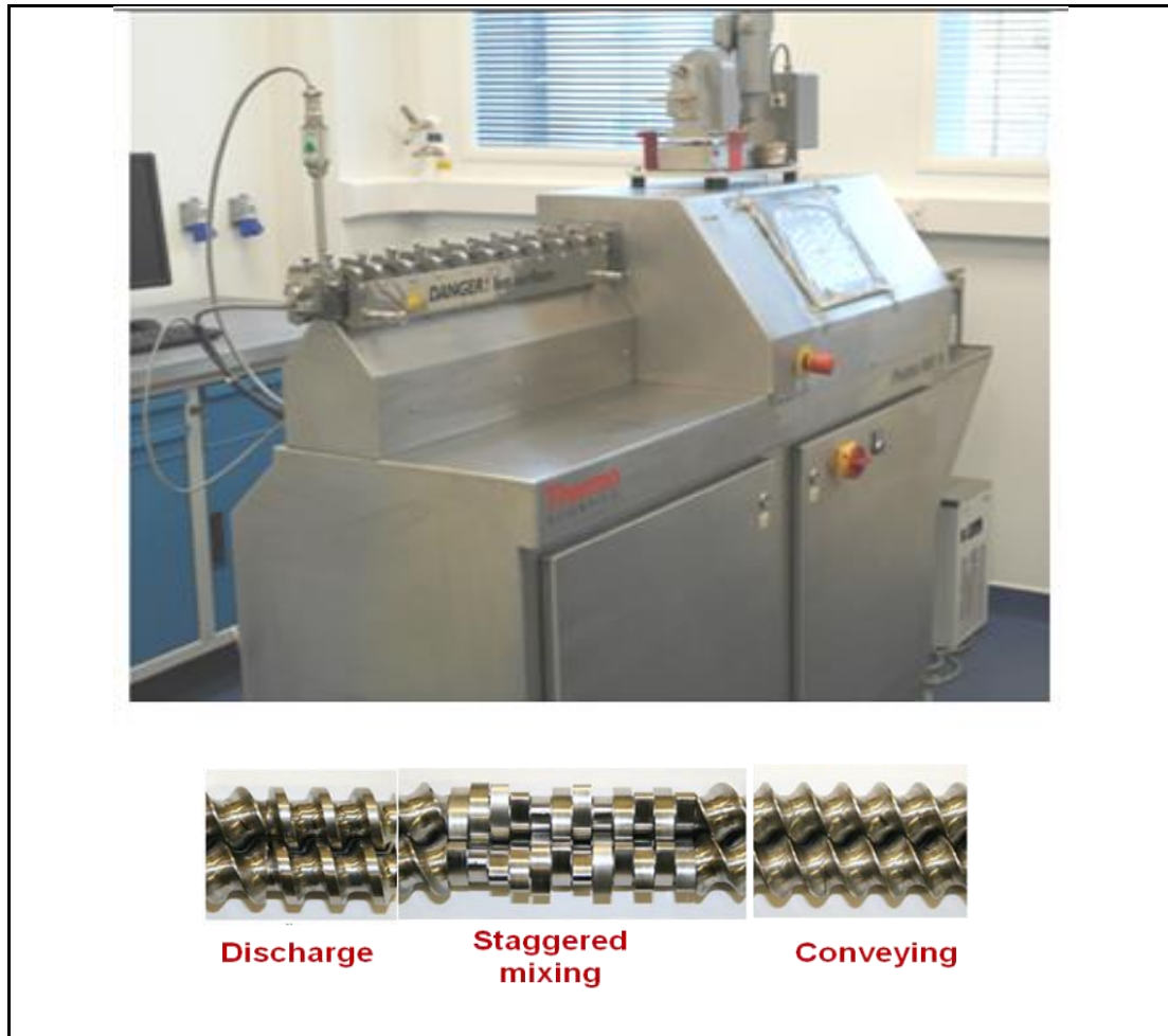
Figure 3.3: Pharmalab HME 16 and screw configuration
