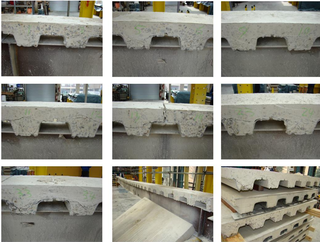
Fig 12 Concrete slab of solid-web composite beam after testing and cutting
