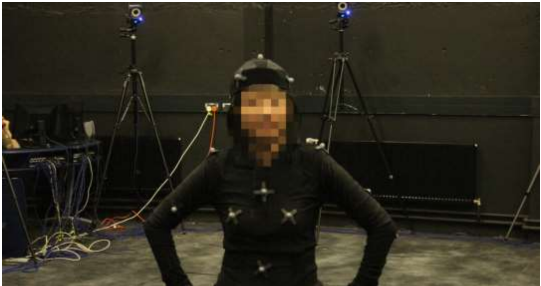
Figure 4: A subject wearing a motion capture suit with motion capture cameras on tripods in the background
