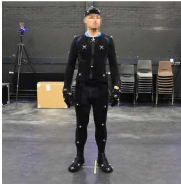
Figure 21: illustrates the marker setup used in capturing the gait cycles in the database
