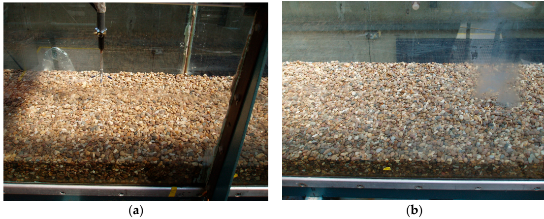
Figure 2. Comparison of (a) water-worked bed and (b) experimentally prepared rough bed in lab flume.
