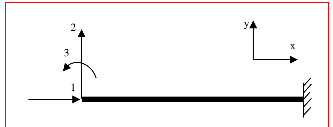
Fig. 4 A cantilever model for computing the relations between the nodal actions and basic deformation parameters
