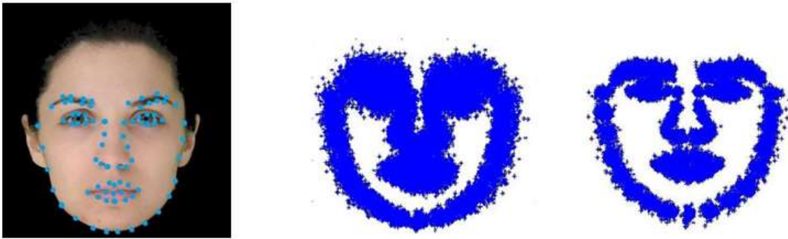
Fig. 1: Face shape captured using landmarks (a) Position of 79 landmarks (b) Unaligned face shapes (c) Shapes aligned using GPA.
