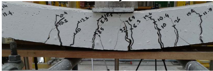
(b) BFRP tensile rupture failure at midspan of SB-125-U slab
