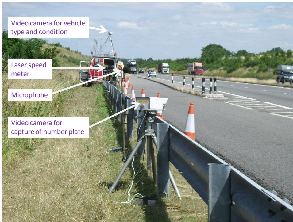
Figure 1: View of measurement set up
