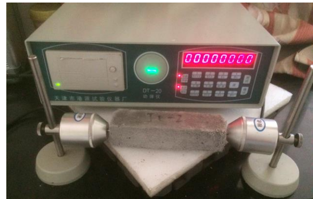
Fig.6 Longitudinal fundamental frequency testing device
