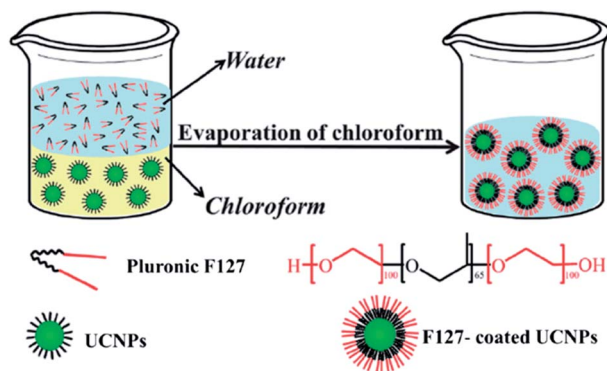
Fig. 4 Schematic illustration of UNCP coating through oil-to-water phase transfer. Reproduced from ref. 45 with permission from The Royal Society of Chemistry.
