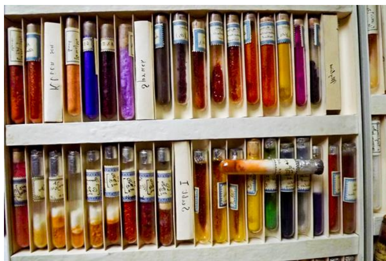
Figure 4. Some of the transition metal complexes synthesis by Werner and his co-workers. Their beautiful colours have long since made them attractive for study and are often useful for characterisation, including identification of coordination geometries, and distinction between isomers. Acknowledgement: Nachlass Alfred Werner, Zentralbibliothek der Universität Zürich.
