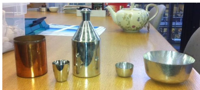
Figure 3. Some of the vessels (including platinum crucibles) used for synthesis in Werner's laboratory. We thank Professor Roger Alberto for his assistance with this photograph.
