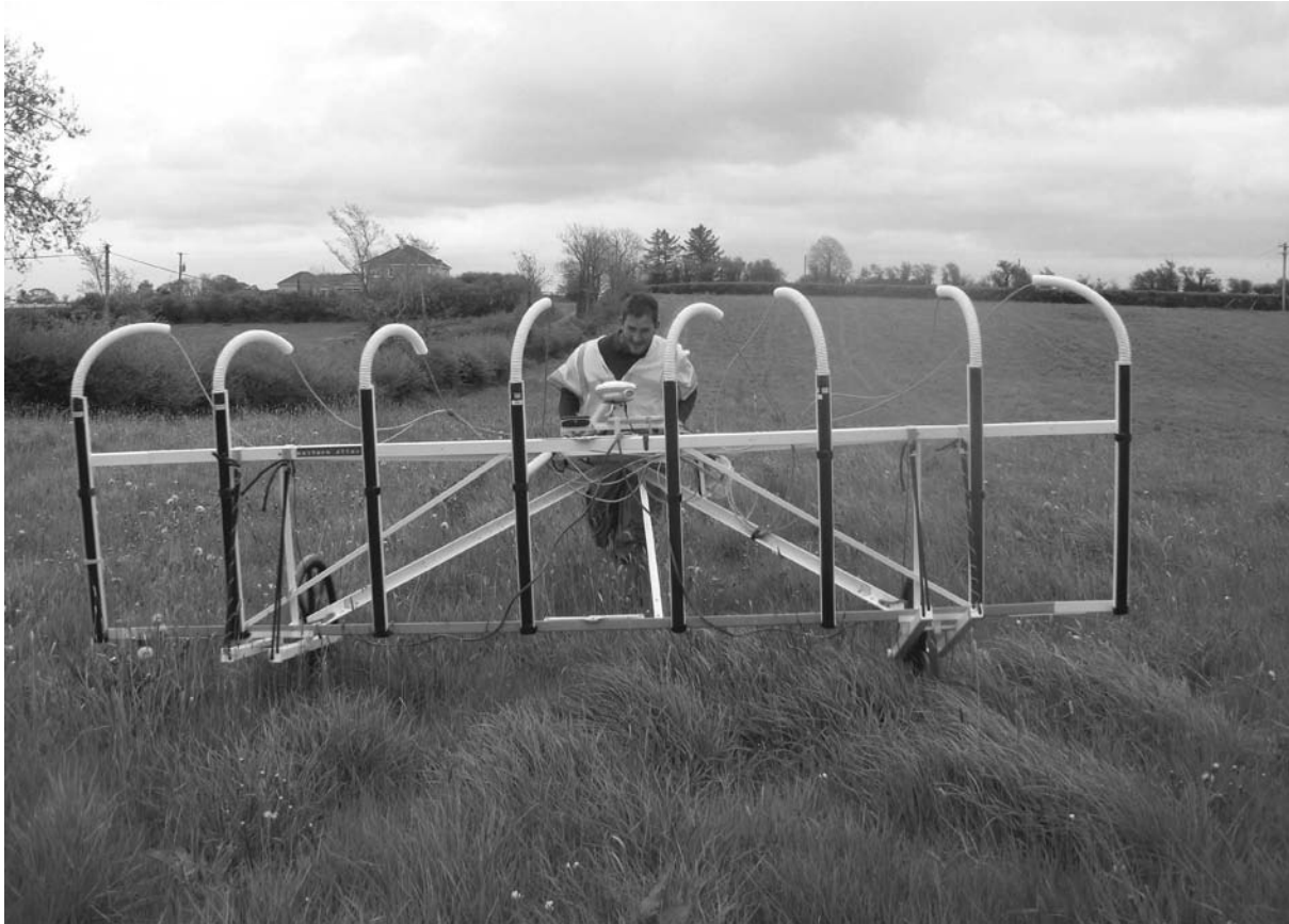
Fig. 2. Multi-sensor cart-arrays are gradually increasing in usage across Ireland. Challenging field conditions – such as rough and poorly drained ground – may preclude some of the advantages offered by ATV-powered arrays, whilst pedestrian-powered carts are extremely useful for the collection of high-resolution data.
