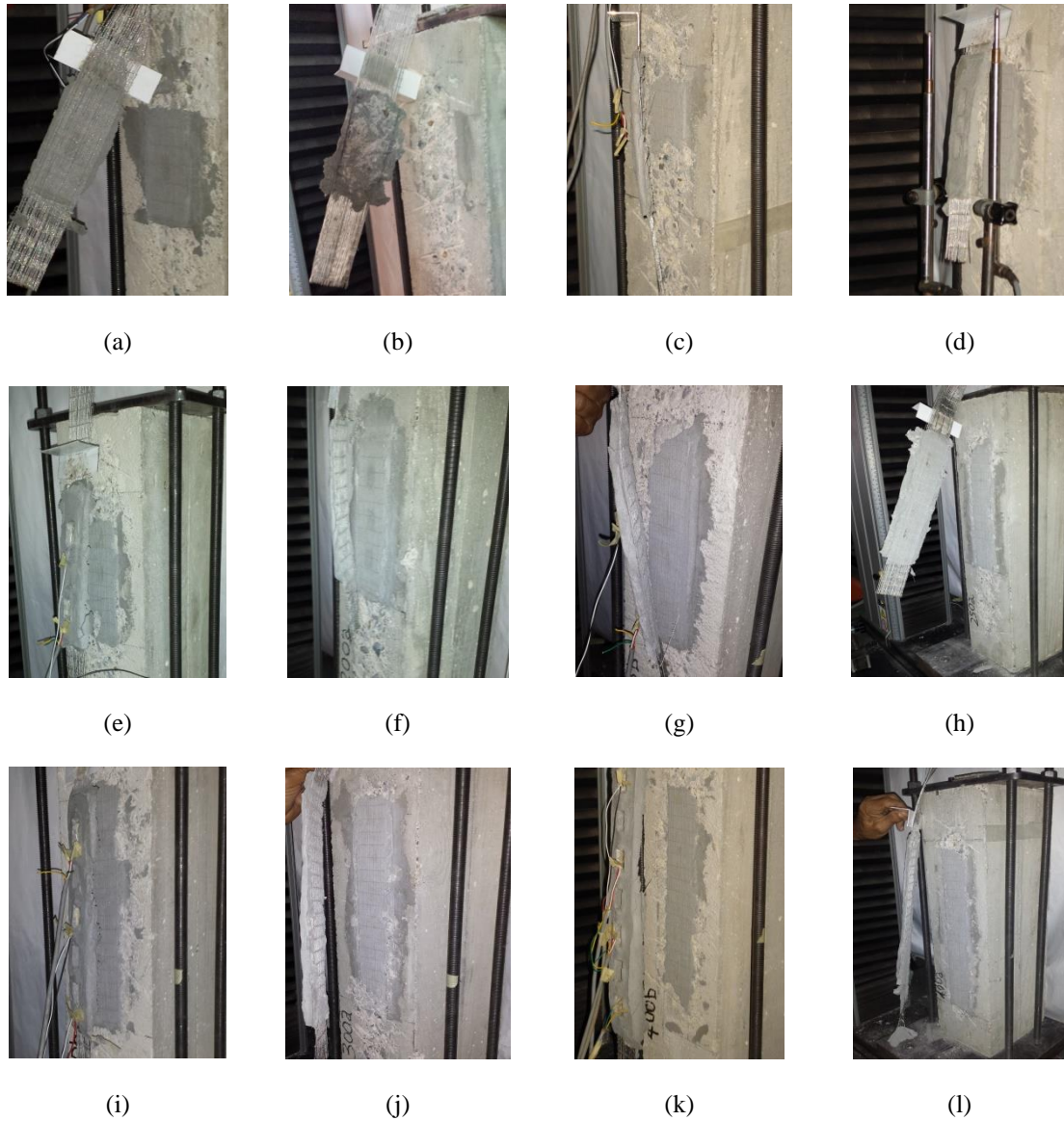
Fig. 7. Failure modes: (a) 100S; (b) 100; (c) 150S; (d) 150; (e) 200S; (f) 200; (g) 250S; (h) 250; (i) 300S; (j) 300; (k) 400S; (l) 400.
