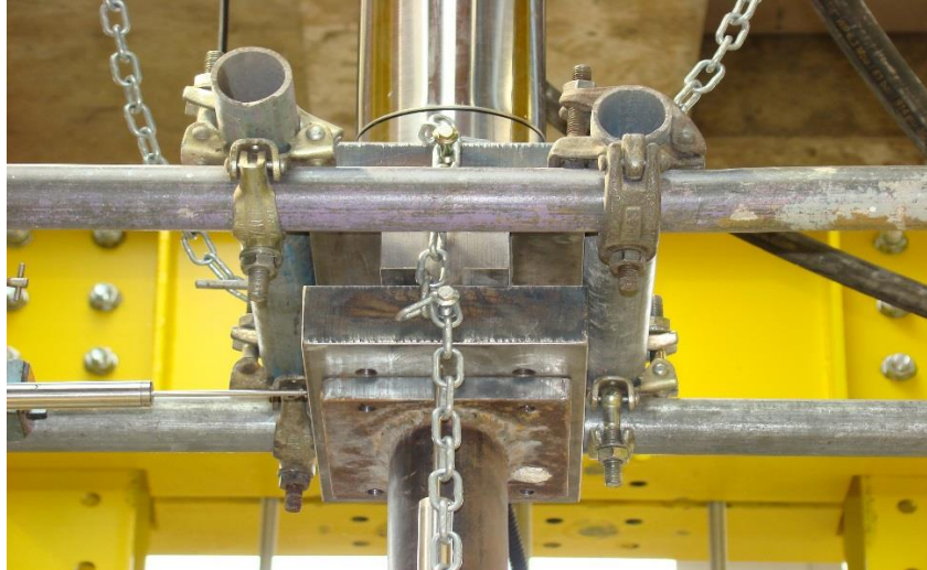
Figure 3. Top plate in contact with the Jack.
