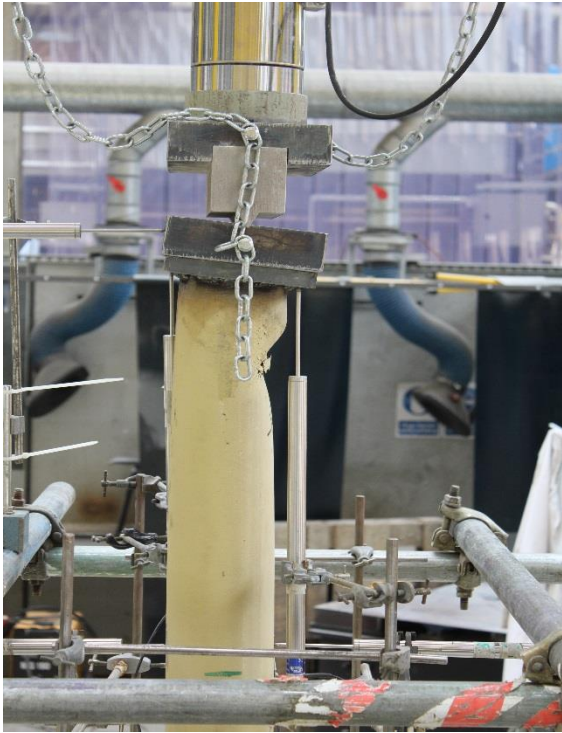
(a) Local Buckling for CII-250-N-2
